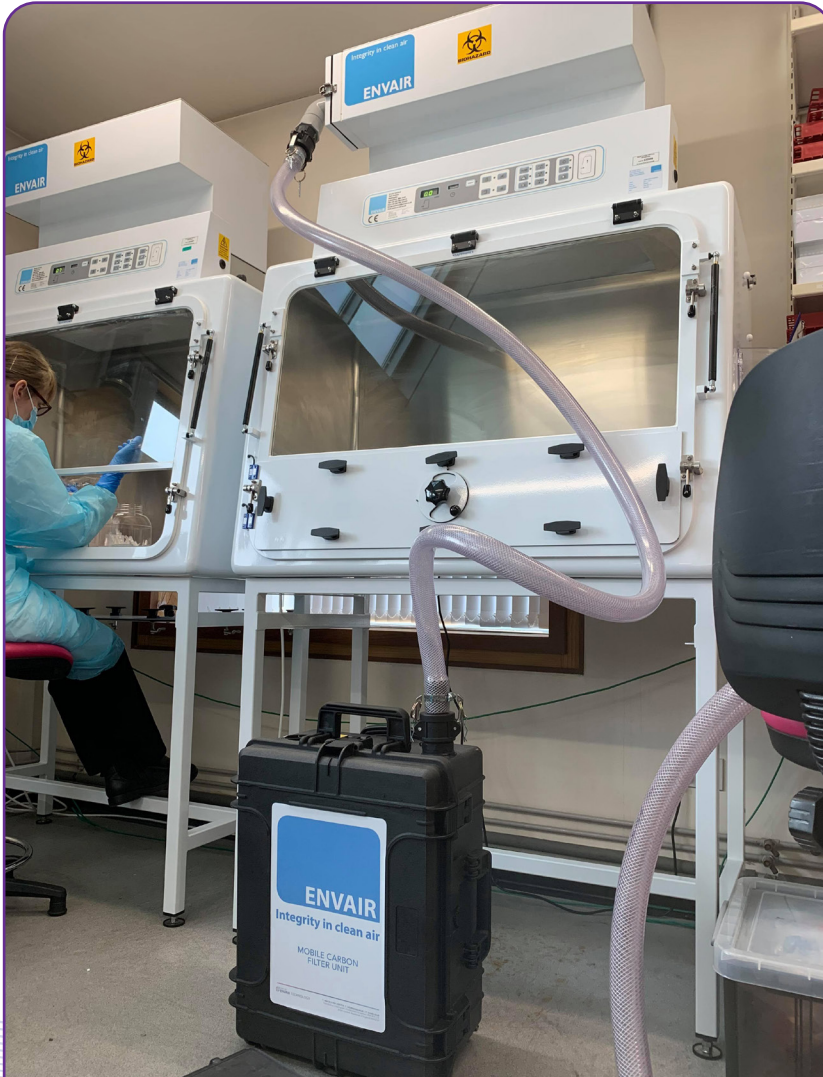
Class I microbiological safety cabinet model Bio 1+ R (recirculating)
