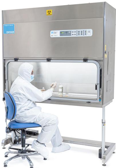
Class II microbiological safety cabinets are designed to allow users to safely carry out manipulations inside the cabinet whilst also keeping the risk of product cross contamination low.
